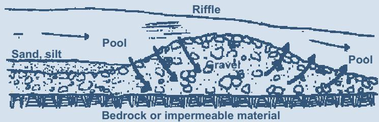
Direction of water interchange between stream and gravel in a salmonid spawning riffle. Where the stream slope increases at the head of the riffle, water flows downward into the gravel. At the lower end of the riffle, where stream slope decreases, flow tends to be upward from the gravel to stream.
